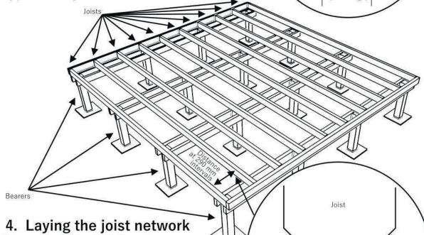
Joists should be laid directly onto your bearers in accordance with the recommended spacing of 250–350 mm. Begin by installing the outside joists to the subframe and continue fixing along the decking bearer network.
